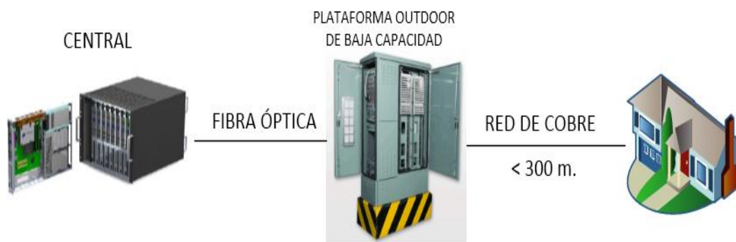
Figura 2.26 FTTC (Fiber to the Curb)
