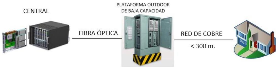
**Figura 2.26 FTTC (Fiber to the Curb)**
