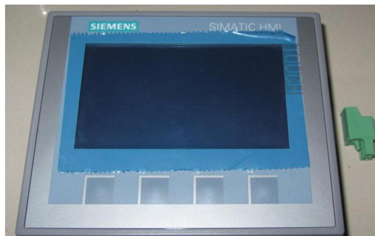
Figura 2.11. HMI KTP 400 Basic
