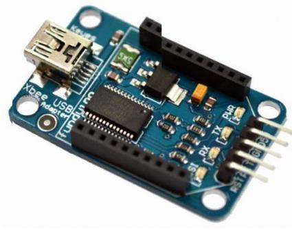
Figura 3.2 XBee EXPLORER USB (*electropro.pe, 2018*)
