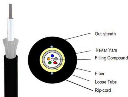
Figura 1.13. Cable central loose tube
