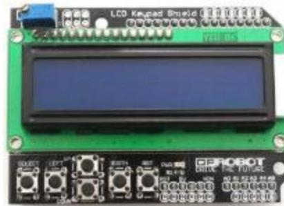
**Figura. 3.20.** Display LCD 16x2 Arduino
