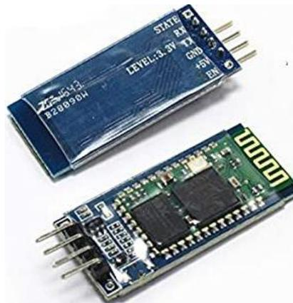
**Figura 1.8** Modulo Bluetooth Arduino HC-05
