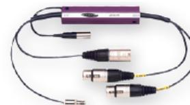
The ASD-771p is a 24 bit/48 kHz analog to digital audio converter. An external reference input allows the output to be synchronised to composite video, AES-3id Digital Audio Reference (DARS) or Word Clock signals. A choice of three full scale levels (+20/+22/+24 dBu) of input signals is possible. The ASD-771p is ideal for audio monitoring and desktop system applications.
