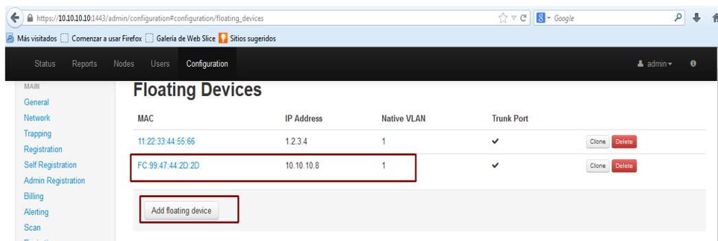
Figura 4.44: ingreso de access point Cisco a PacketFence
