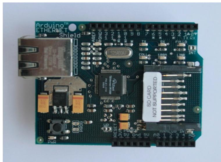
**Figura 2.4.** Arduino Ethernet Shield<sup>16</sup>
