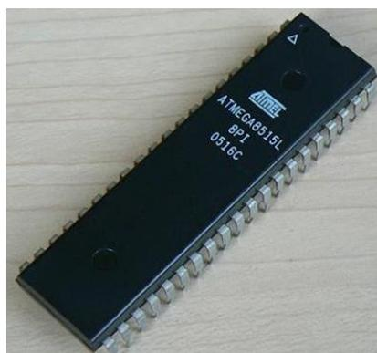
**Figura 2.16:** Microcontrolador AVR.<sup>27</sup>
