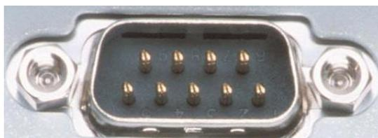
Figura 2.13: Puerto serial DB9 macho.<sup>23</sup>
