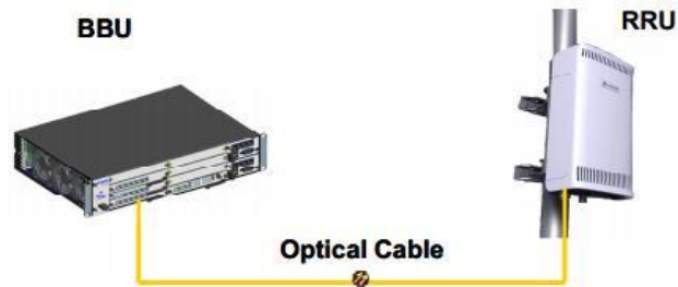
Huawei DBS3900 LTE System Architecture
