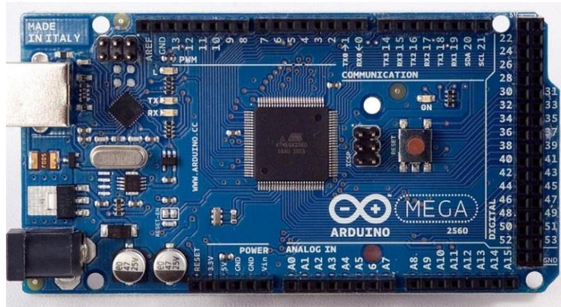
**Figura 5.** Arduino mega 2560
