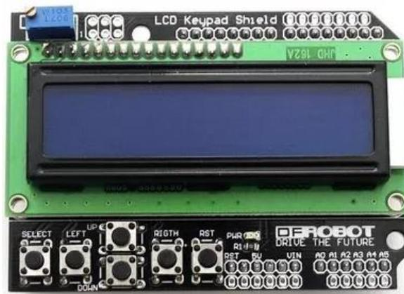
Figura 1.14 Módulo shield keys lcd (Oscar, 2013)
