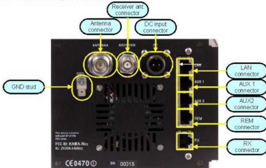
Figure 3-2, Rear view, transmitter unit, TA-7650/25/10.
