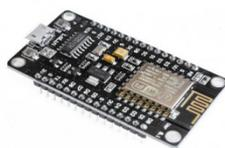
**Figura 4.** NodeMCU
