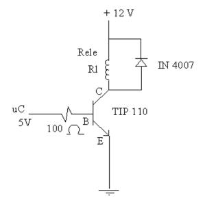
Fig 3.11 transistor
