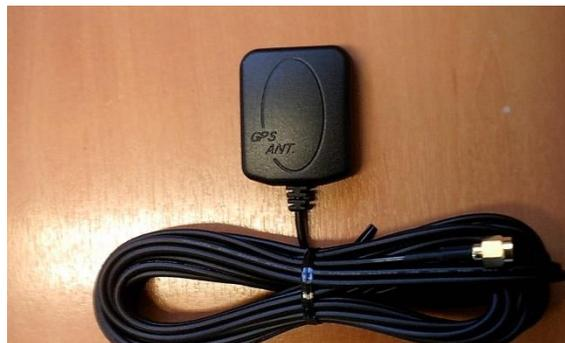
Figura 2.12: Antena GPS AT-65
