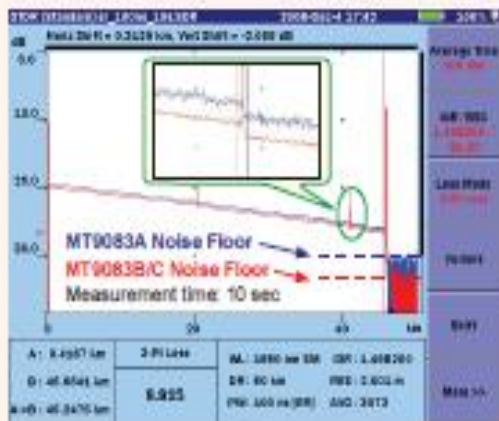
Fig. 2: Improved measurement range from MT9083A to MT9083B/C (100 ns shown)
