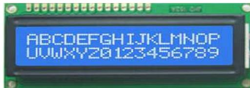
Figura 2.14. Display LCD 2x16<sup>11</sup>
